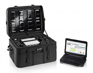
Using the unique design formula of AirShip, CP Cases produced a case to fulfil the specification precisely. AirShip comprises typically a rugged textile outer covering allowing for branding, straps, handles and fasteners, foam internals which are cut to the design of the equipment and reinforced honeycomb polypropylene for strength. In addition CP Cases added lid hinges, that could be fixed whilst testing is undertaken, and wheels with telescopic handles for ease of handling.
